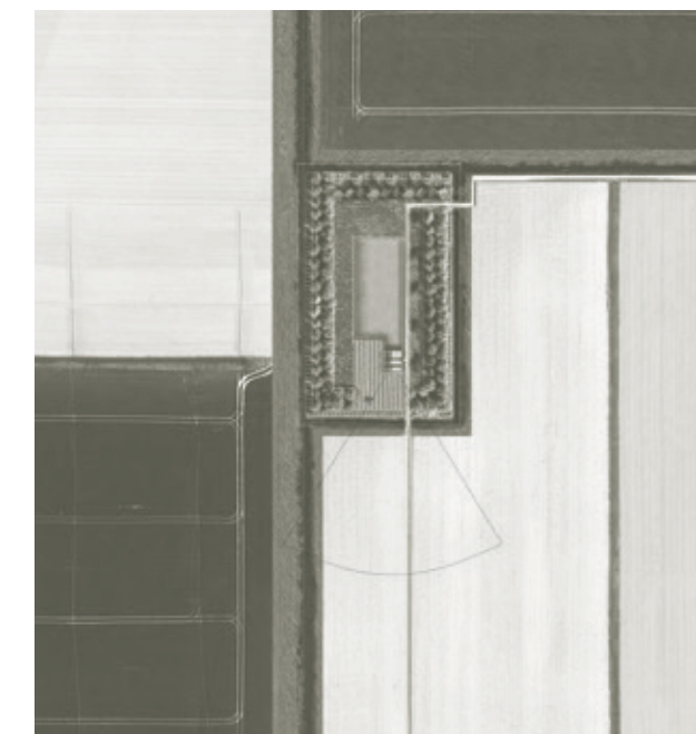
Plan of former farmyard where the barn has been replaced by a lower infiltration area for rainwater.
